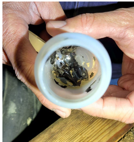
Fig 1: Metal fragments pulled from gearbox
